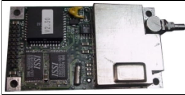
Figure 1. The Conexant Jupiter GPS Receiver (-391) With Right Angle SMB RF Connector (Top View – Shown Approximately Actual Size)
